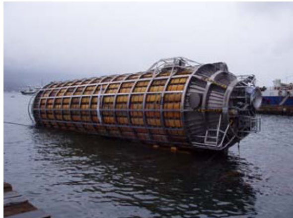
Figure P-2. An aluminum shuttle being towed to the Prestige site.
